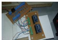
Fig. 1: Adaptation stage with two ADS1115 converters
