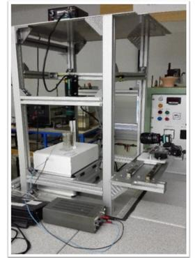
Fig. 1: Electrolytic cell & main experimental setup
